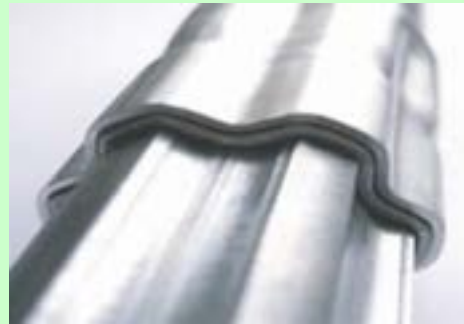
Example of magnetic pulse welding / forming
