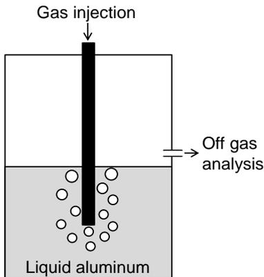
Simulation of gas-liquid reactions in exp. setup
