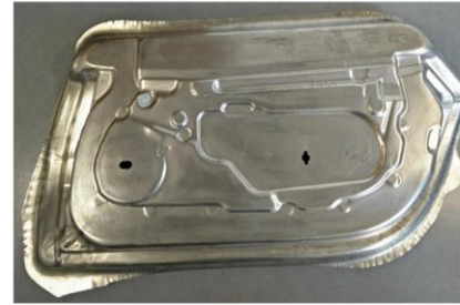
HFQ ® Heat Treatment Forming and cold-die Quenching system for high-strength aluminium alloys
