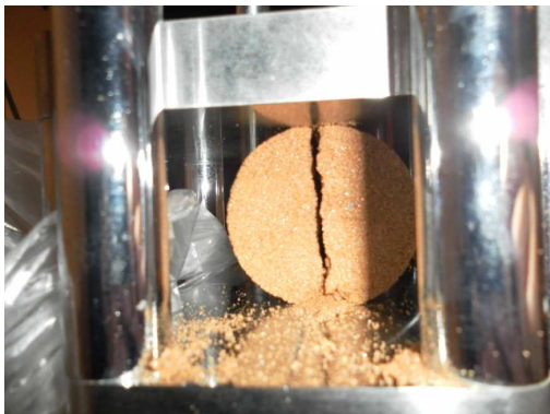
Brittle material at lower temperature
