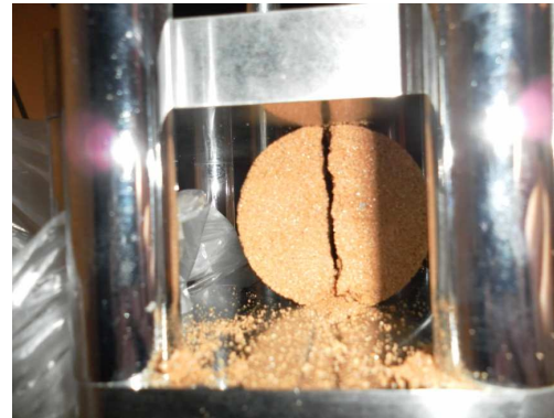
Indirect tensile test
