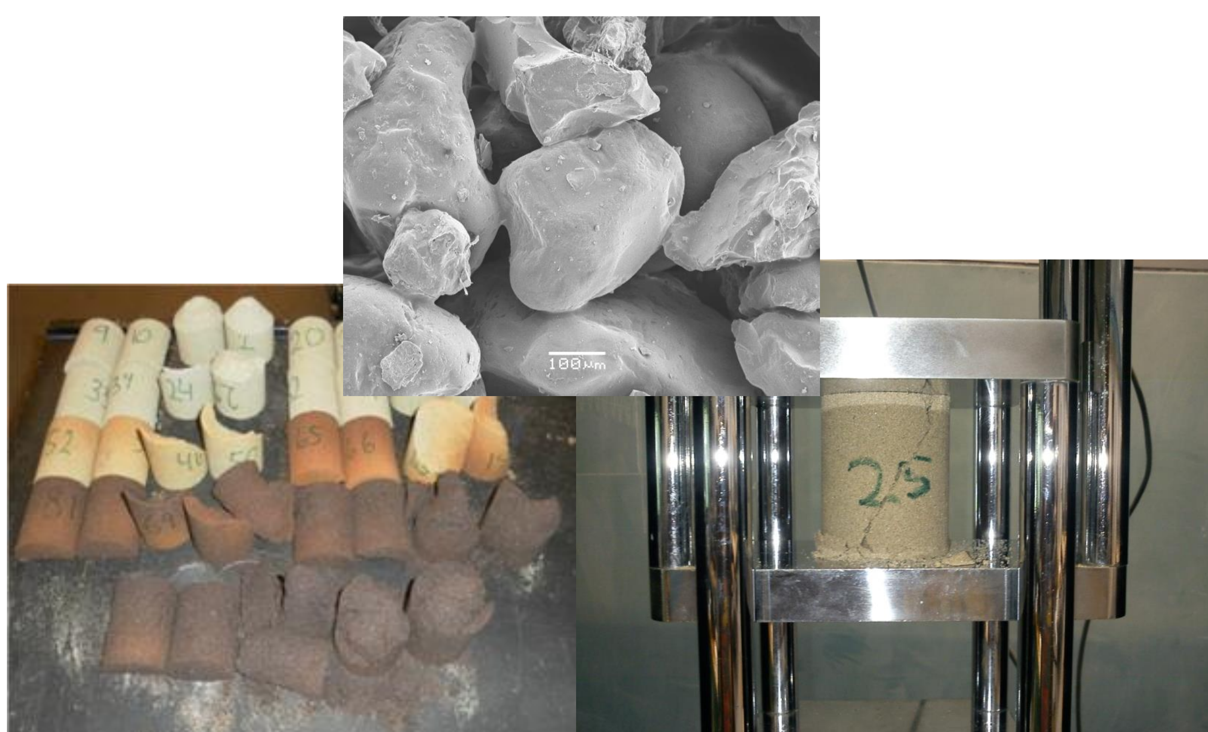
Figure 2: Characterization of various sand/binder systems at increasing temperatures using several different measurement methods.
