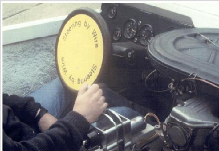
Sidestick with potentiometer and rotary magnet
