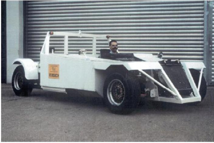
Research vehicle at ika 1991 with electro hydraulic Steer-by-wire system
