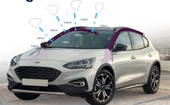
Form blow hardening of tailor rolled tube
